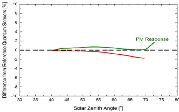
Mean **cosine response** of seven Apogee SQ-500 quantum sensors. Cosine response was calculated as the relative difference of SQ-500 quantum sensors from the mean of replicate reference quantum sensors (LI-COR models LI-190 and LI-190R, Kipp & Zonen model PQS 1). The red data are AM measurements; the green data are PM measurements.
